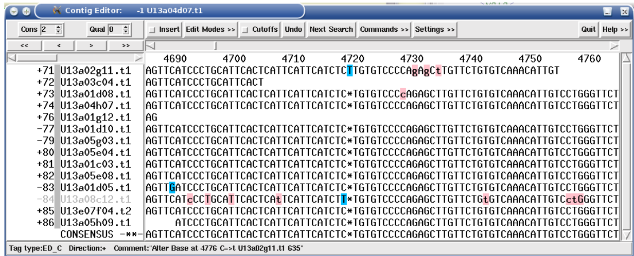
Figure 1.7: Sanger assembly with EdIt automatic editing routines. Bases with pink background are corrections made by EdIt after assessing the underlying trace files (SCF files in this case). Bases with blue background are base calling errors where the evidence in the trace files did not show enough evidence to allow an editing correction.
